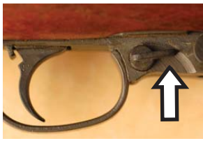
An M1 Carbine with the safety engaged or "on." This safety is disengaged by rotating it clockwise.
